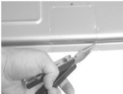
FIGURE 11 REMOVING CONDENSATE KNOCKOUT
